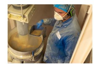
Milling whole herbs and spices such as pepper, cardamom and fenugreek into powders at various mesh sizes from 500 micron to 8mm
